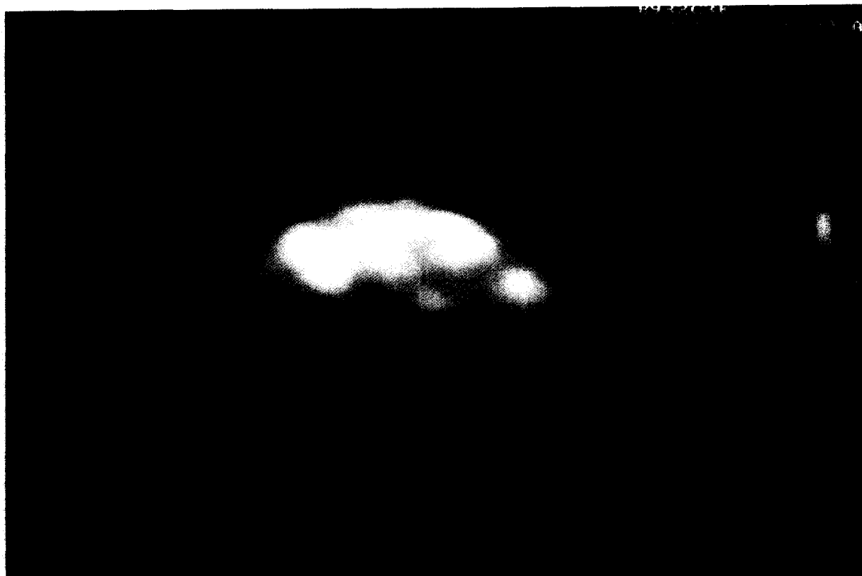
Fig. 6. PSTM three-dimensional image of a group of nanospheres made from \beta CD- C_6 with a diameter of 147.7 nm by vertical measurement. Topography image, 5 \mu m xy scan.
