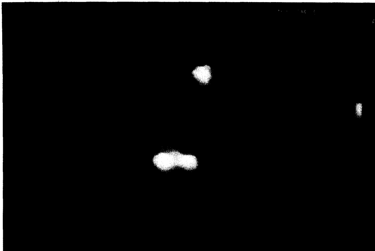
Fig. 7. PSTM three-dimensional image of a group of nanospheres made from \beta CD- C_6 with a diameter of 147.7 nm by vertical measurement. Topography image, 2 \mu m xy scan.
